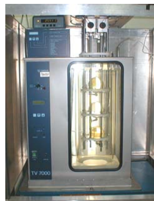
Fig. 2. Hydrostatic Weighing System. Thermostatic bath with the national density standards in the top and in the bottom and the sphere under test in the middle.
